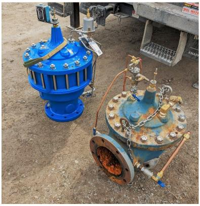
New PRV (left) and old PRV (right)
